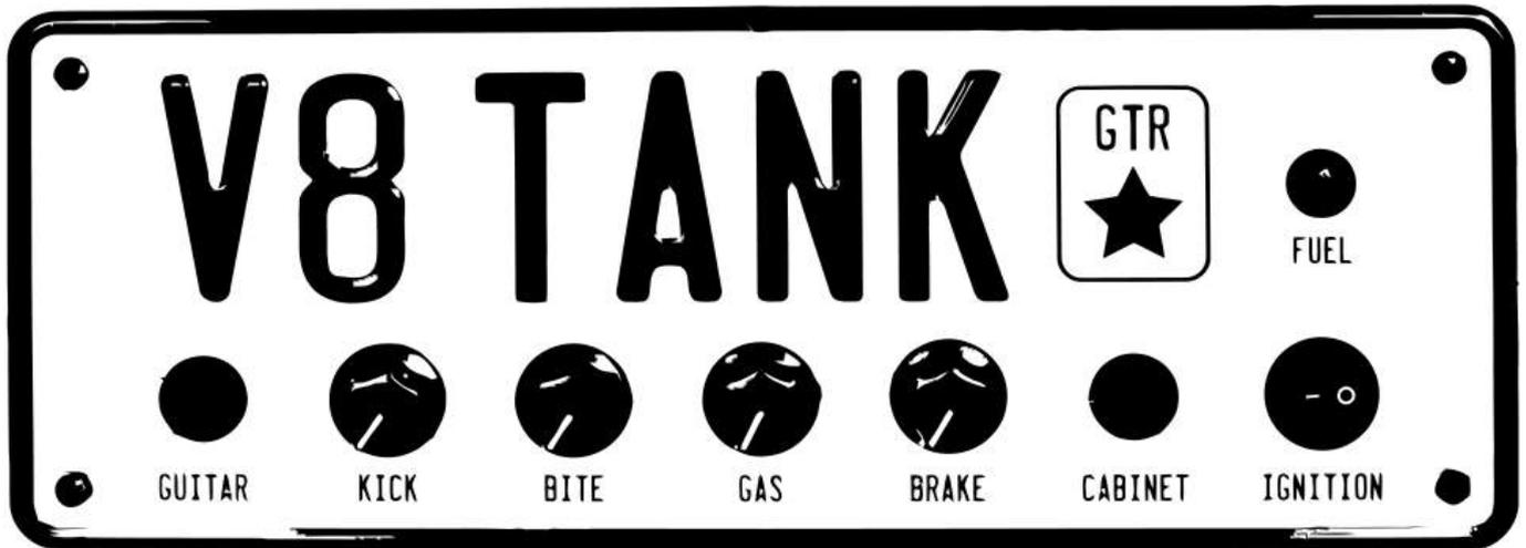
**GUITAR** · Input for connecting guitar or other instruments. This is a stereo jack that has been wired to contain both clean and overdrive options. By inserting plug in only half way you will get a cleaner sound.
